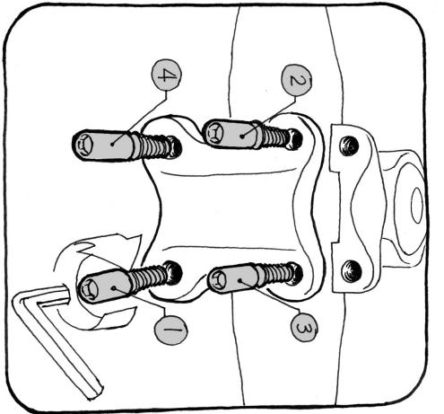
Working in an "X" pattern, tighten each of the bolts about 1/4 turn per pass to keep the tension even.
