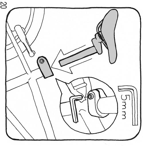
Loosen the seat post clamp bolt if necessary. Slide the seat post into the seat tube. Position the saddle so that it is approximately the same height as your child's hip and tighten the seat post clamp to secure.
