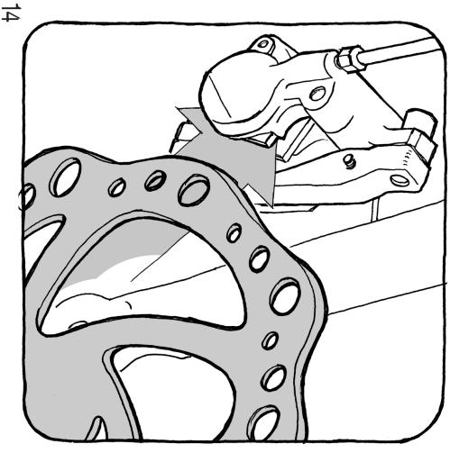
The ROTOR should slide in between the pads of the brake, easily.
